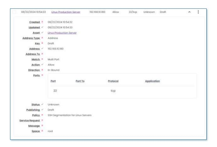
For the last step of the Enforcement process, we must now disable the default Linux allowall firewall rules so that only the connections permitted by our segmentation policies are allowed:
